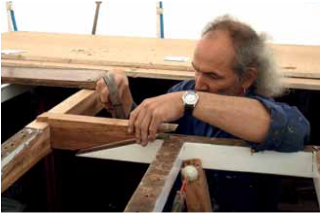
Above left: Scarphing in a new deck piece Above right: Her stern area needed a lot of work
